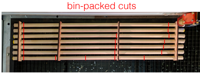
Figure 2: We pack all of the rod-lengths into a single cut plan over a small number of raw rods. Rods are positioned in place using a “comb” jig with holes cut at regular intervals matching the spacing of the automatically generated cut plan.
